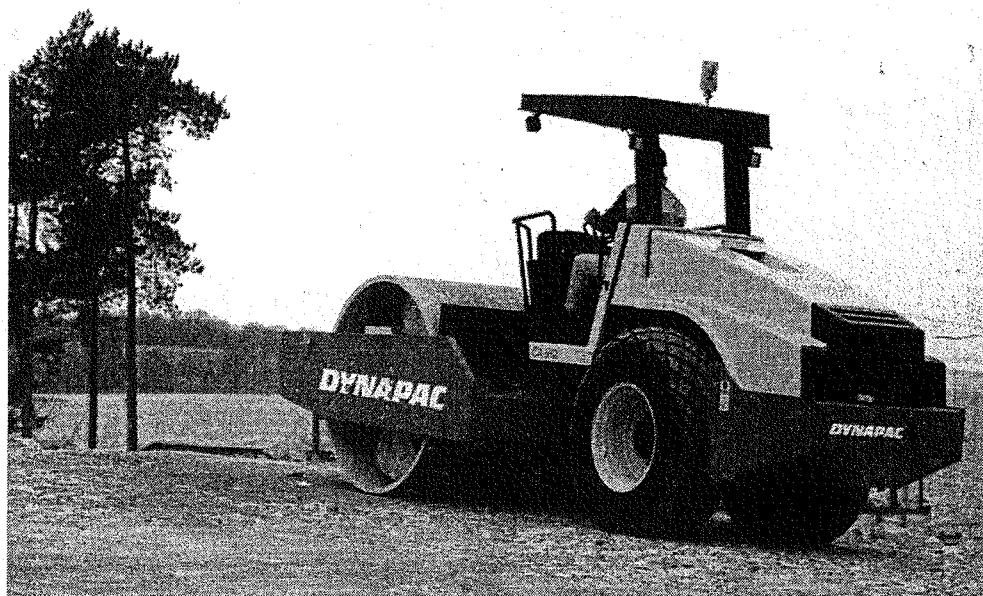
FIGURE 5.14 Vibratory roller (photograph courtesy of Dynapac, Inc.).
