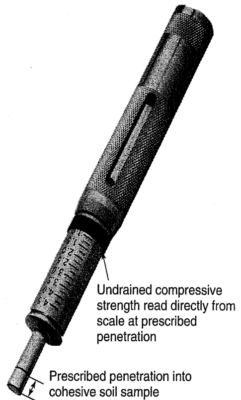
FIGURE 12.43 Pocket penetrometer, a hand-held device which indicates unconfined compressive strength (photograph courtesy of Soiltest, Inc., Evanston, Illinois).
