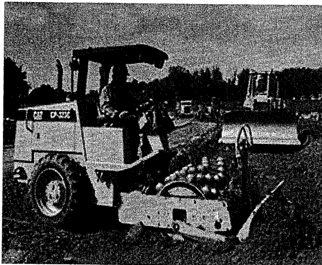
FIGURE 5.11 Self-propelled sheepsfoot roller (photograph courtesy of Caterpillar Inc.).
