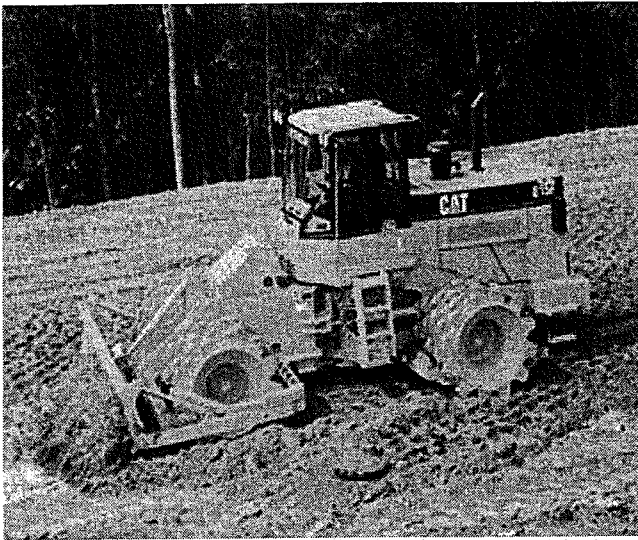
FIGURE 5.12 Self-propelled tamping foot compactor (photograph courtesy of Caterpillar, Inc.).
